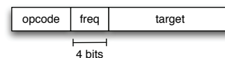
Figure 5. Branch-on-random instruction format. Instead of encoding an explicit condition for the branch, a branch-on-random specifies a frequency (a 4-bit field in our implementation), which is converted to the probability that the branch should be taken using the formula: (\frac{1}{2})^{freq+1} .
